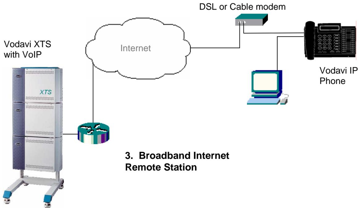
When using the Internet for access to the XTS system, quality of service cannot be guaranteed. The use of a hardware Virtual Private Network (VPN) may be necessary to ensure adequate voice quality and priority for voice traffic.
