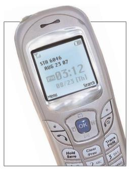
points placed throughout your site. The handset can automatically "hand-off" a signal among these access points, allowing, for example, warehouse staff to provide immediate and direct customer service while performing their regular duties throughout the warehouse.
